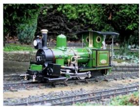
**Peter Angus** has recently sent us the above photos of one of his latest delightful models. This is built as a gas fired live steam locomotive in 16mm/ft scale for 32mm gauge track and based on Sharp Stewart works number 3016 delivered in 1882 to the Darjeeling Himalayas Railway as their No 9. The photographs were taken by **Geoff Munday**. I'm sure you will remember the NBL Burma Mines loco from Peter in 2010 and we look forward to seeing more great work from him in the future.
